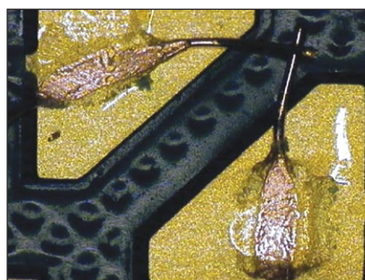
0.005 in (0.127 mm) diameter magnet wire to gold pad
