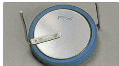
Battery tab welding
