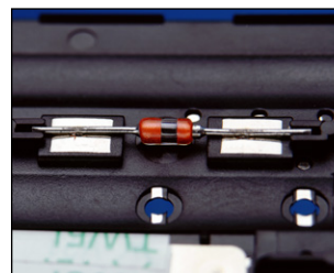
Welding components to leadframe
