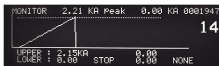
Monitor Screen – Shows weld current exceeding limit.
