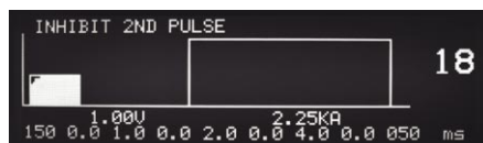
Run Screen – Shows that 2nd Pulse was inhibited from firing.
